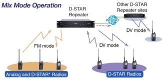
\* D-STAR radio can receive both FM and DV mode signals.
